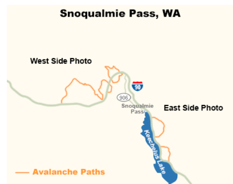
Snoqualmie Pass WSDOT avalanche control areas.
